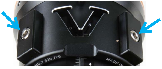
9. Draw Tube Holder Screws
